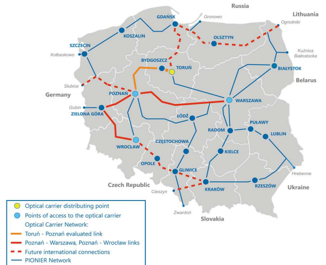
Fig. 1. National optical carrier signal distribution system as part of the NLPQT project based on dedicated optical fibres of the PIONIER network.
